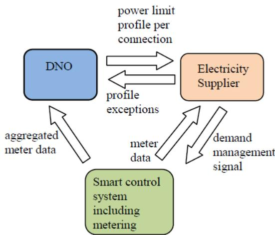
**Figure 2 Proposed process for joint DNO/supplier demand management - Paper 0289**
