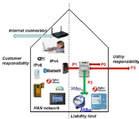
**Figure 7 - The Data Flow Interface - Paper 0668**
