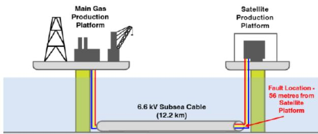
**Fig. 2:** from paper 1334 – Subsea circuit overview
