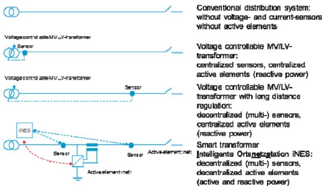
**Fig 18:** from paper 1332 – Systematic of smart grid concept
