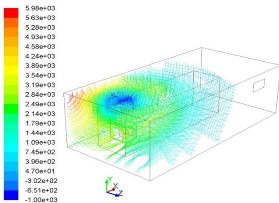
**Fig. 30:** from paper 1301 – CFD simulation showing a pressure peak in the corner of the switchgear room 17 ms after the fault initiation
