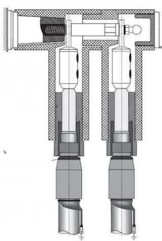
**Fig. 10:** from paper 1288 – Cross-section of two stacked, unscreened connectors with integrated earthing bolt
