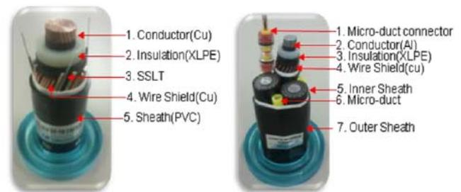
**Fig. 24:** from paper 0951 – Composite cables design and configuration of cable joint
