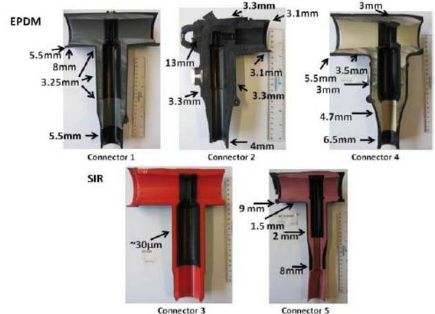
**Fig. 7:** from paper 1341 – Section of the connectors illustrating their design
