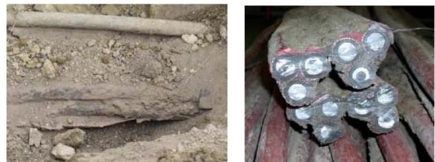
**Fig. 5:** from paper 0651 – Melted cables and dry soil around
