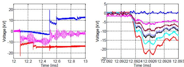
**Fig. 12:** from paper 0412 – Energising of a transformer under no-load: voltage traces at the terminals of winding (red and blue), mid-point (pink) and 4 end disks, showing internal resonance and capacitive voltage distribution between the turns
