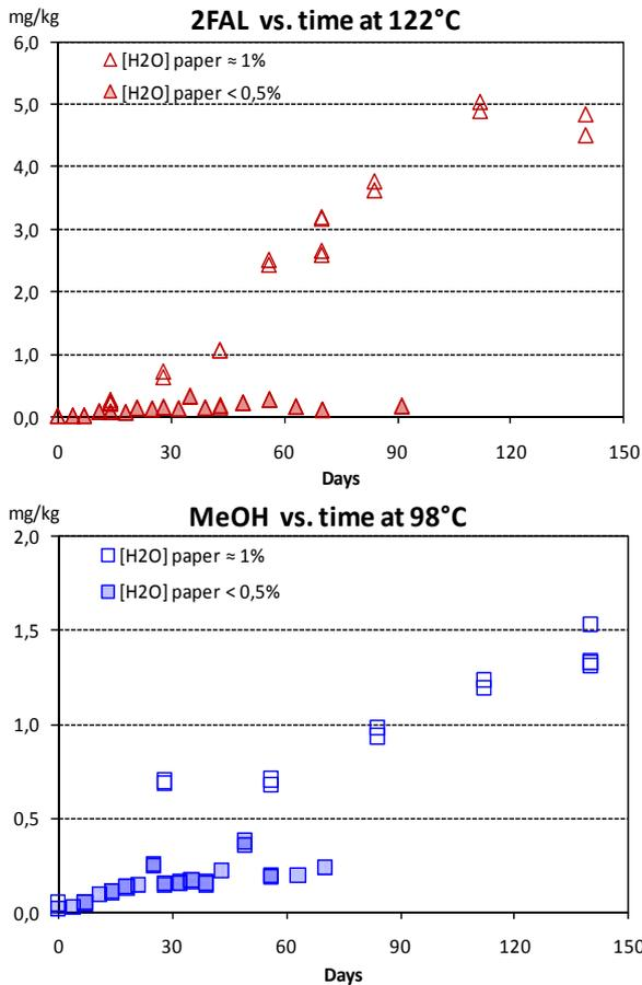
**Fig. 8:** from paper 0407 – Evolution of the 2-FAL at 122°C and MeOH at 98°C (in ppm) with different initial levels of water content in the paper
