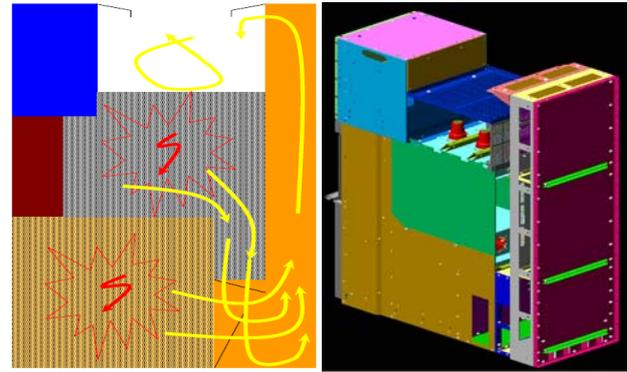
**Fig. 31:** from paper 1057 – Example of introverted release in case of internal arc fault
