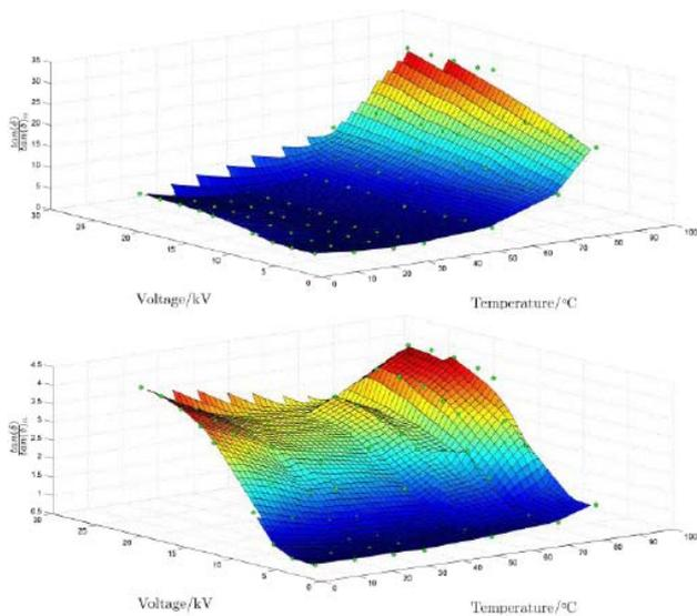
**Fig. 4:** from paper 1258 – Tan( $\delta$ ) fingerprints of a sample that has been in operation for over 40 years (top) and of a sample that has been in operation for over 20 years (bottom)
