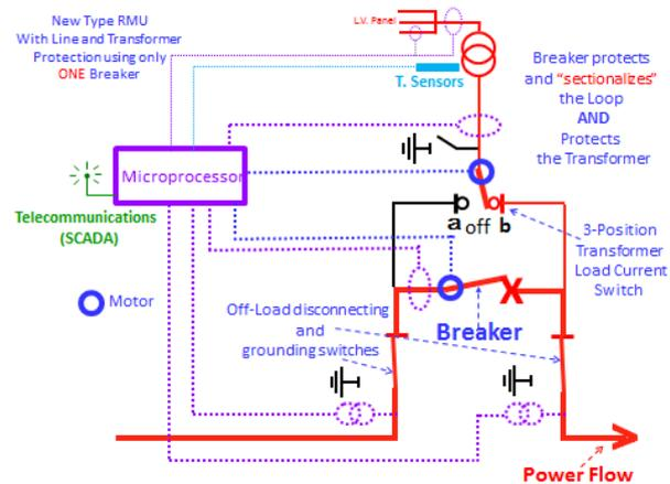
**Fig. 33:** from paper 0274 – Single line diagram of “smarter RMU”
