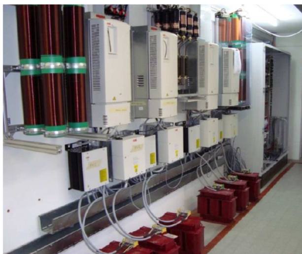
Fig. 15: Principle scheme and view of components used to emulate prosumers and feeders in the Gridlab units.
