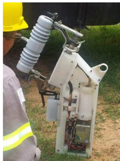
Fig. 24: Recloser prototype before installation
