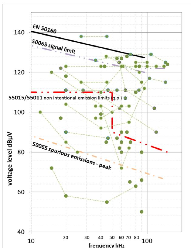
Fig. 3: Emission levels measured at different sorts of equipment, from 40 devices compared with limits for non-intentional emissions and signals as well as PQ levels in present standards
