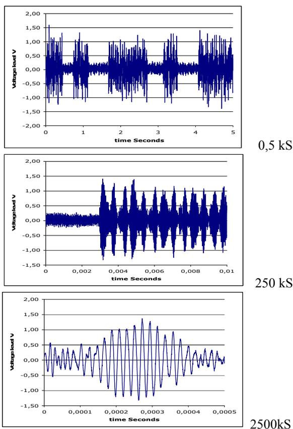
Fig. 2: Example for discontinuous signal of an AMR-PLC system
