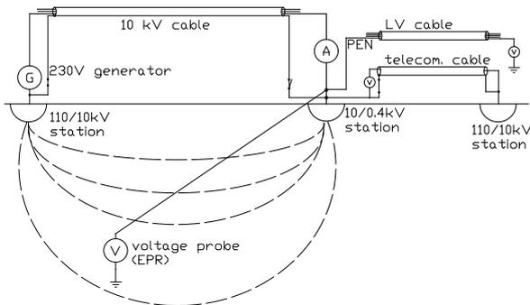
**Figure 1:** Illustration of the electrical circuit for the low voltage grounding measurement
