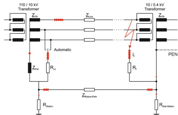
**Figure 2:** Simplified illustration of the earth fault localization method “short time earthing of an additional healthy phase” [15]
