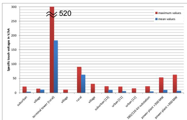
**Figure 3:** Typical measured specific touch voltages in different areas [10]
