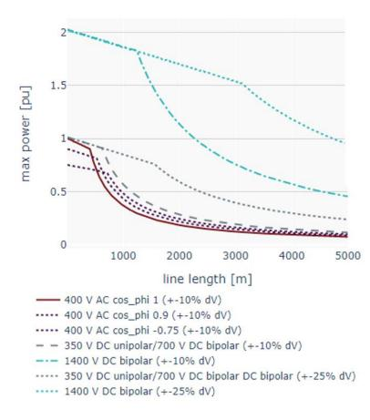
Maximum transmission power vs line length; cable type XAY2Y 4x150; max 1400  $V_{DC}$  bipolar; p.u. of max. power at 1m line length operated at 400  $V_{AC}$ ,  $cos(\varphi) = 1$ .
