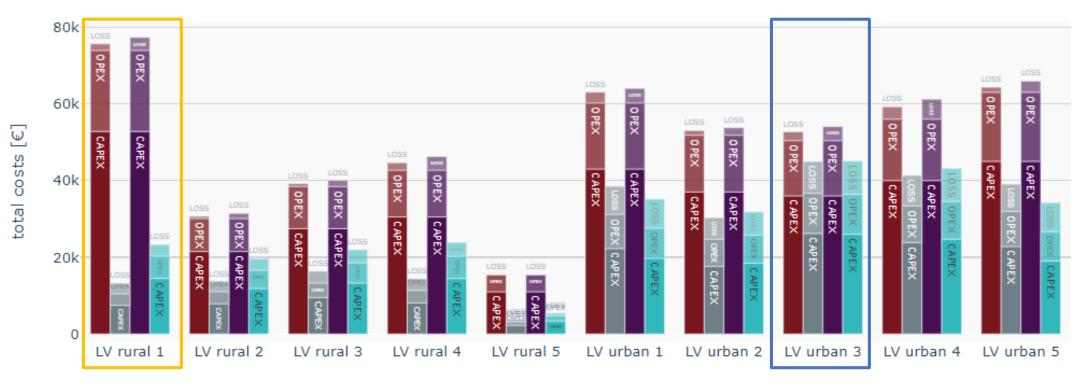
Comparison of TOTEX costs for AC grid reinforcement and conversion to DC for all LV feeders in test grid, TOTEX divided in CAPEX and OPEX (losses costs (LOSS) are indicated separately from the rest of OPEX costs) using calculation parameter from Table 5 in paper and yearly simulation results.
