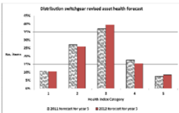
Fig. 1: The evolution of distribution switchgear health index forecast as in Paper 490
