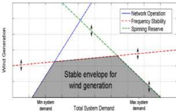
**Fig. 1.16: Stable envelope for wind generation operation on Shetland (UK) power system (paper 1381).**
