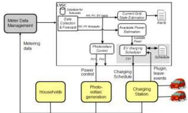
Fig. 2.5: Low Voltage Grid Controller architecture (paper 1268).
