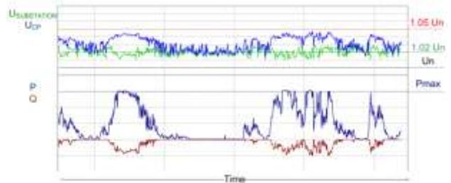
**Fig. 2.8: DG voltage control (regulating Q) with droop and deadband (paper 0494).**
