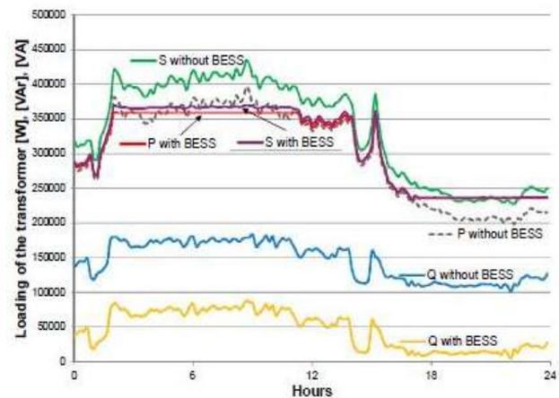
**Fig. 4-5: Peak shaving through battery energy storage system (BESS) (paper 1172).**
