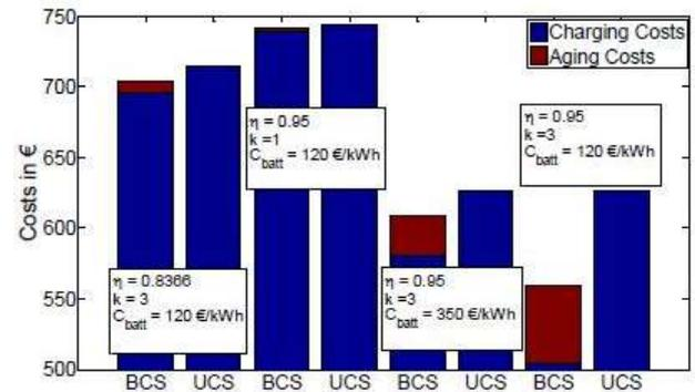
Fig. 3-5: Cost comparison between unidirectional (UCS) and bidirectional (BCS) charging strategies (paper 0661).
