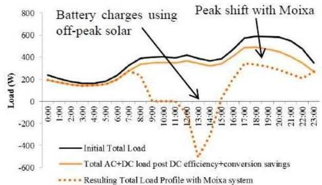
**Fig. 4-3: Peak load management through DC/storage system (paper 0797).**
