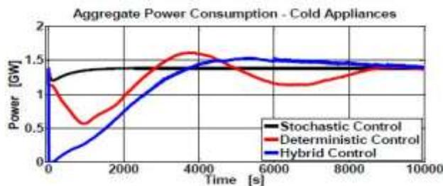
Fig. 3-3: Power consumption of dynamic demand appliances after a system disturbance (paper 0435).
