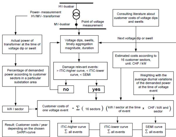
**Figure 29:** Elements of the Power Quality cost model to estimate the customer costs for dips and swells [B4-0255(CH)]
