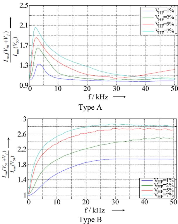
**Figure 3:** Type A and Type B behaviour of CFL tested with a two frequent voltage (50 Hz nominal +  $V_{HF}$ ) showing the current ratio as a function of the frequency of  $V_{HF}$  [B2-0999(DE)]
