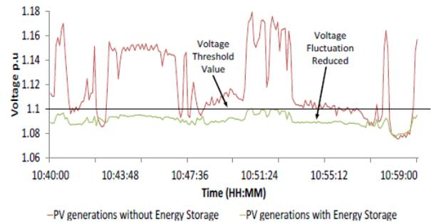
Figure 18: Voltage rise reduction by energy storage at time, summer day [B3-0504(UK)]
