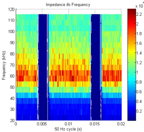
**Figure 5:** Periodic impedance analysis on a digital TV decoder showing very low impedance during periods of conduction of the diode rectifier [B2-1435(BE)]
