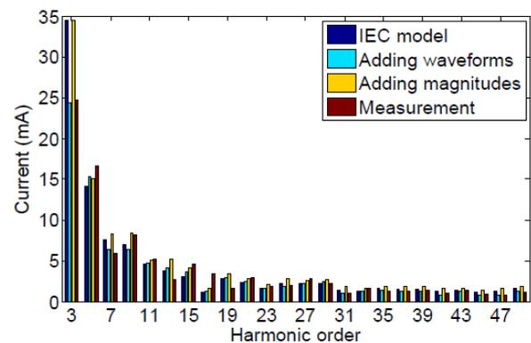
**Figure 7:** Different approaches for the aggregation of harmonic emission from 2 different LED street lamps [B2-0291(ES)]
