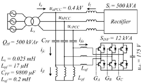
**Figure 8:** Hybrid active parallel filter topology for harmonic filtering and reactive power compensation (passive part 500 kVAR, active part 12 kVA, [B2-0763(SI)])
