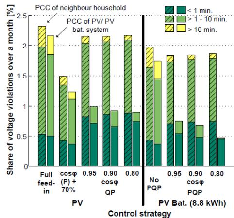
Figure 19: Voltage violations at the PCC of the neighbour household and at the PCC of the PV/ PV battery system for different control strategies [B3-1396(DE)]
