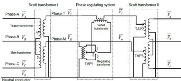
**Figure 22:** The diagram of the proposed voltage balancing system [B3-0246(UK)]
