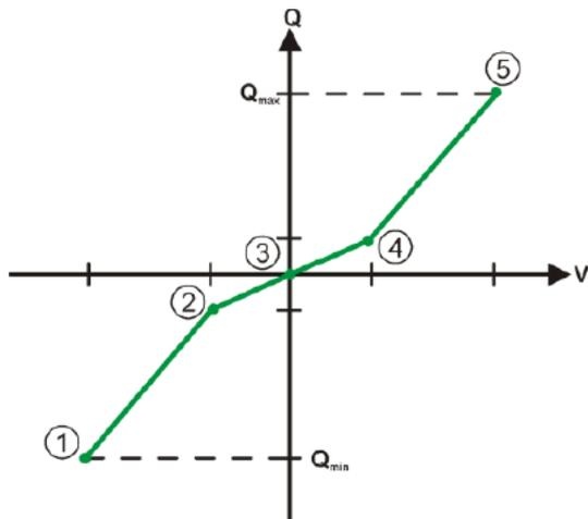
Figure 17: Example for Q-V-control curve [B3-0644(DE)]
