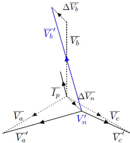
**Figure 21:** Phasor diagram of the three-phase voltage at the end of the feeder [B3-1303(BE)]
