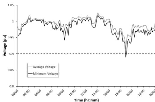
**Figure 16:** Voltage and current profiles for a household showing an example of the minimum voltage falling below the lower permitted limit of 0.9 pu [B3-0674(IE)]
