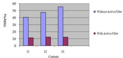
**Figure 10:** Harmonic current before and after the installation of the parallel active filter in an automobile company [B2-1372(IR)]
