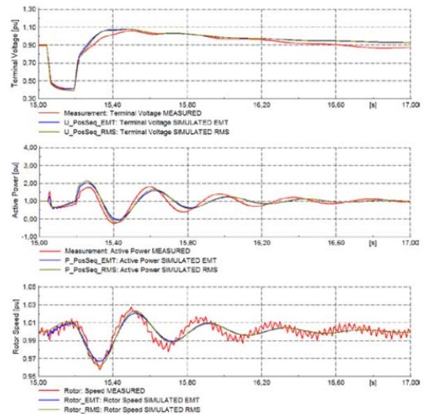
**Figure 25:** FRT of a 5.5 MVA / 10.5 kV gas-engine-driven generator; voltage dip lasting 150 ms [B3-0260(AT)]
