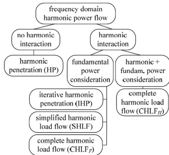
**Figure 12:** Classification of harmonic power flow methods [B2-1262(DE)]
