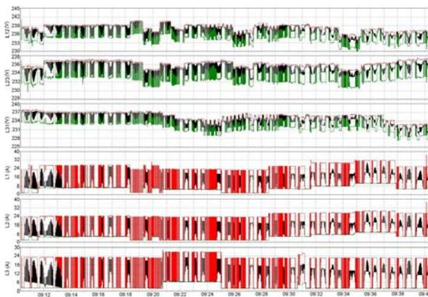
**Figure 23:** Very frequent load changes (red/black current), and voltage changes (green/black) due to tankless water heater in a residential home [B3-1302(NO)]
