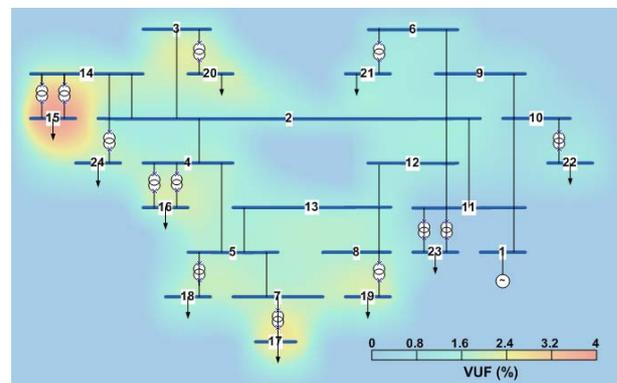
Figure 20: "Heat map" of the network indicating the areas affected by unbalance [B3-0530(UK)]
