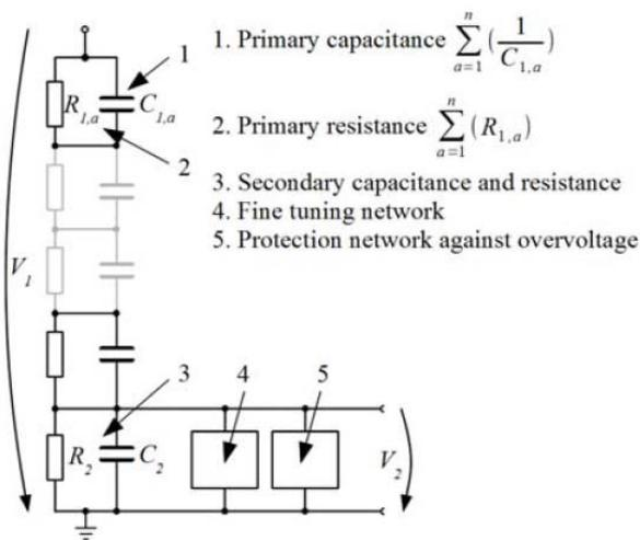
**Figure 6:** Electric circuit diagram of the RC-divider according to [B2-0195(CH)]
