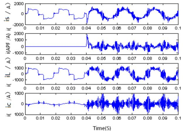
**Figure 9:** Simulation results according to [B2-1128(CN)] illustrating resonance problems of SAPF for compensation current-type harmonics with normal method, where,  $i_s$  grid current;  $i_{apf}$  compensation current,  $i_L$  load current,  $i_c$  current of the shunt capacitor branch
