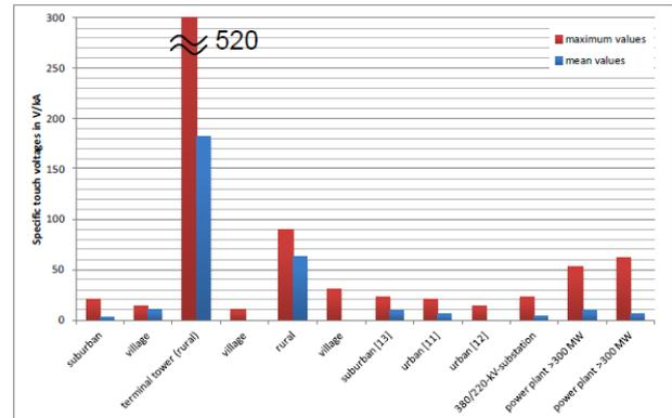
**Figure 2:** Typical measured specific touch voltages (V/kA) in different areas [B1-0035(AT)]
