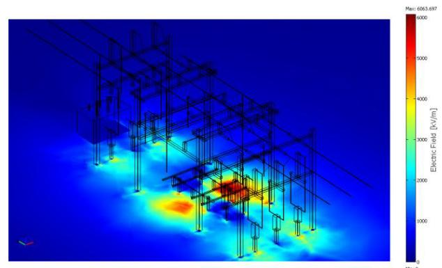
**Figure 1:** Distribution of the electric field on a plane situated at a height of 1.5 m in relation to substation patio, perspective view [B1-1298(BR)]
