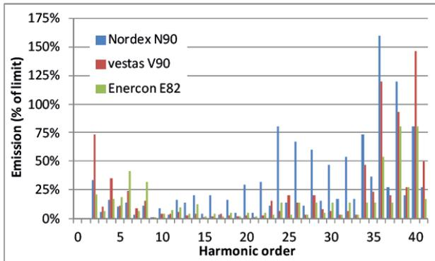
**Figure 11:** Emission spectra from 3 modern MW-class wind turbines as a percentage of the IEEE 519 limits [B2-0408(SE)]
