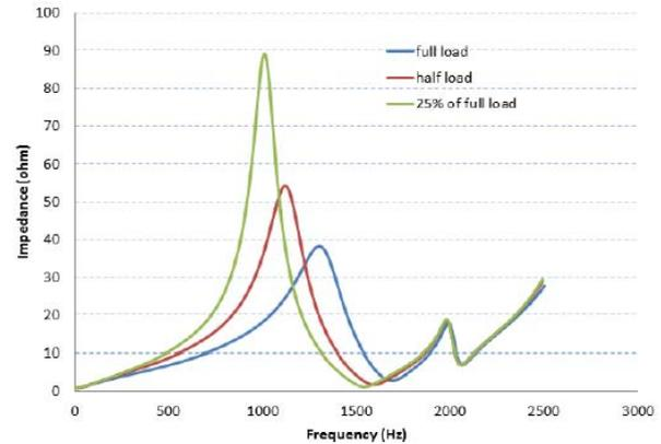
**Figure 14:** Simulation of the impedance spectrum for different loading situations according to [B2-0256(NL)]
