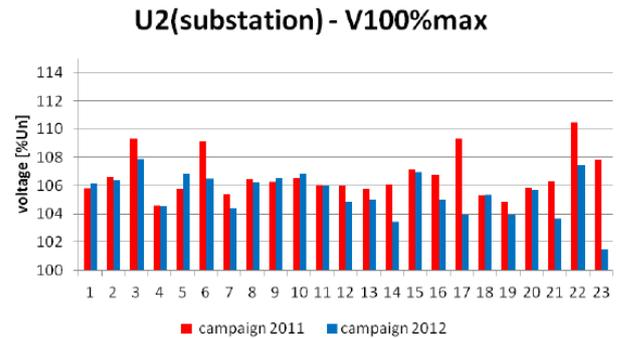
**Figure 27:** Evaluation of maximal 10 min RMS values of supply voltage in 23 LV grids during week measurements [B4-0024(CZ)]
