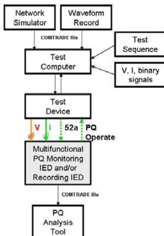
Figure 26: Test system block diagram [B3-1362(US)]
