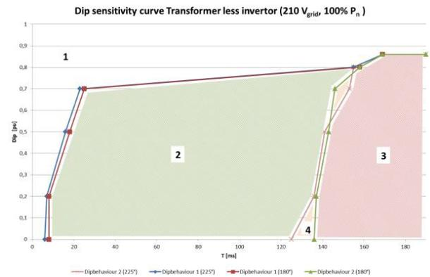
**Figure 24:** Example voltage tolerance curve, (1) normal operation, (2) disconnection and automatic reconnection, (3) ‘hard’ disconnection, (4) uncertainty range due to starting point of dip within cycle [B3-1009(BE)]
