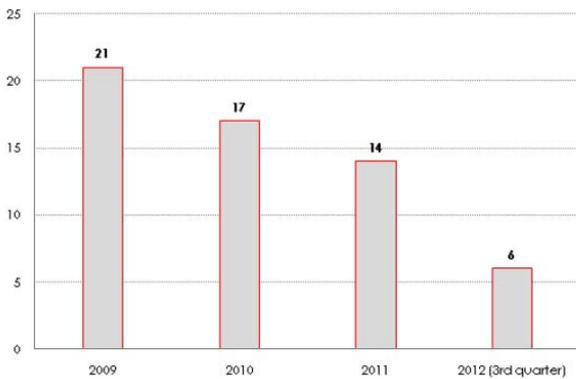
**Figure 13:** Reduction of the 5<sup>th</sup> harmonic voltage in the Portuguese network due to measures to reduce resonances; weeks not in accordance in 5<sup>th</sup> harmonic are shown [B2-1289(PT)]
