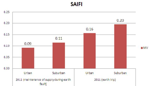
**Figure 30:** Improvement of SAIFI index by using a shunt circuit-breaker in underground cables (maintenance of supply during earth fault) according to [B4-0112(CH)]
