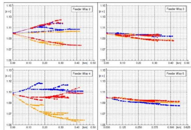
**Figure 15:** High Generation Voltage-Distance Plots ( $V_{Grid}=1.06p.u$ ) [B3-1481(UK)]
