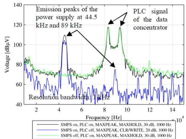
**Figure 4:** Conducted disturbances in PLC caused by the switching frequency of a power supply [B2-1391(FI)]
