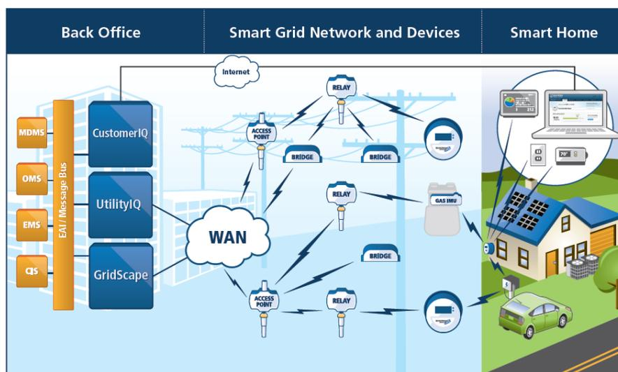
Figure 4—22: RF Mesh Smart Grid architecture
