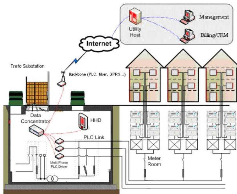
Figure 4—11: PLC Prime reference architecture
