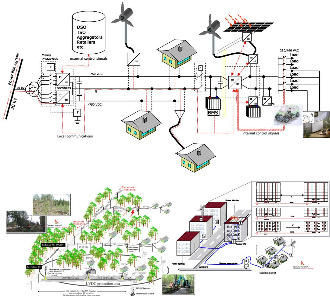
**Figure 4—32: Principles of LVDC-based electricity distribution system. Basic equipment structure a) and examples of applications b)**
