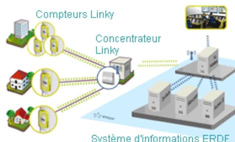
Figure 4—17: ERDF Linky system architecture
