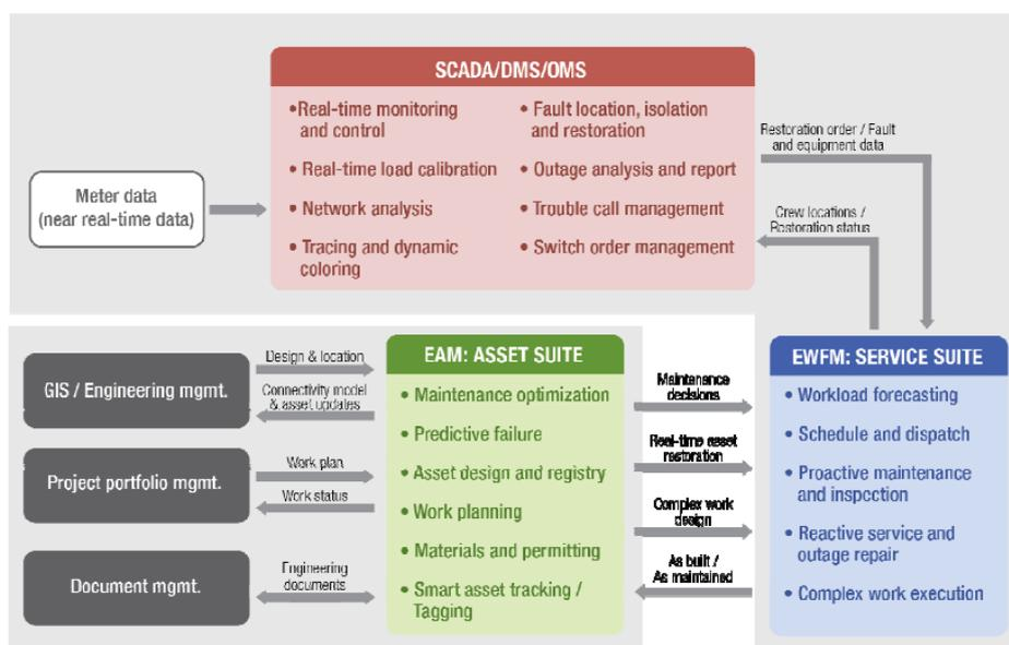
Figure 4—40: Typical Smart Grid data management architecture (Source: Ventyx)
