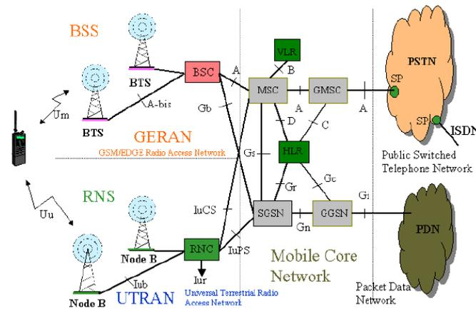
**Figure 4—23: Mobile network operator infrastructure**
