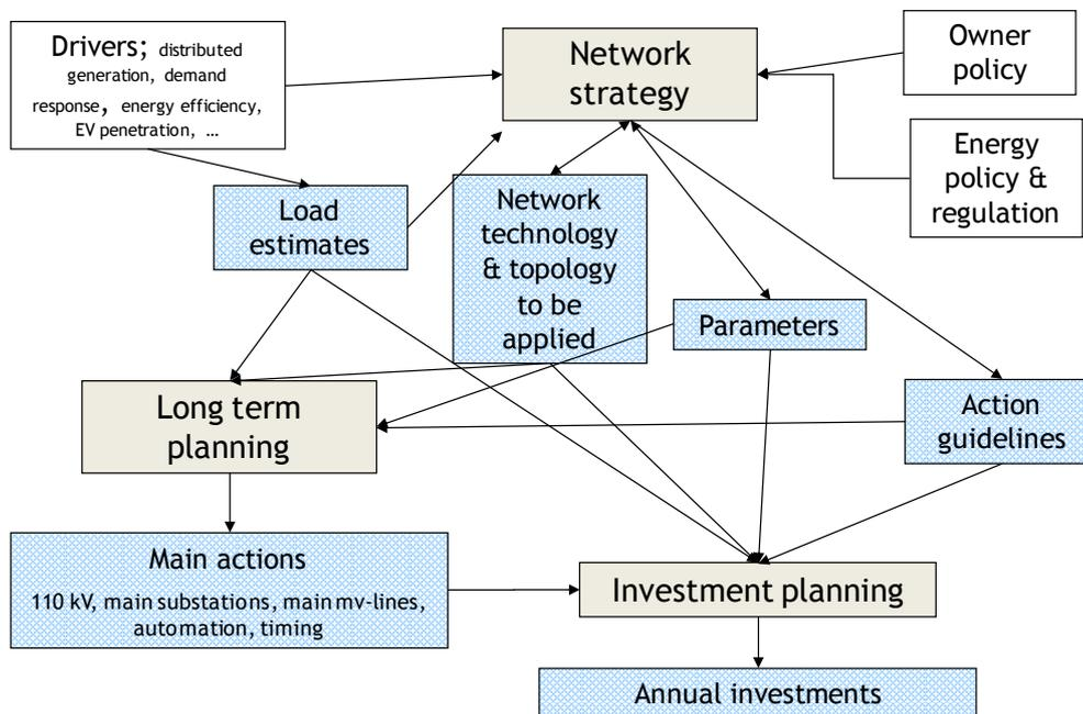
Figure 4—31: Planning process in the grid development
