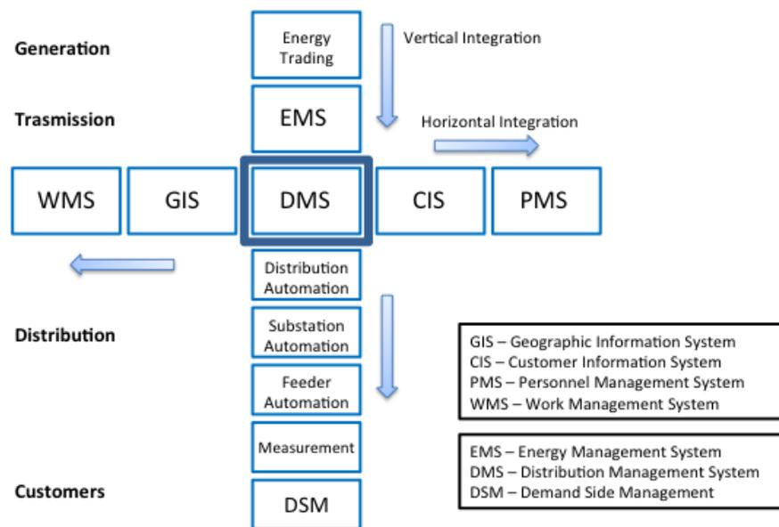
Figure 4–3: Vertical and Horizontal integration of a DMS
