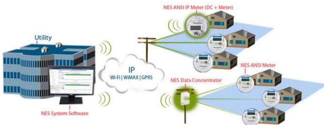
Figure 4—14: Network Energy Service system architecture
