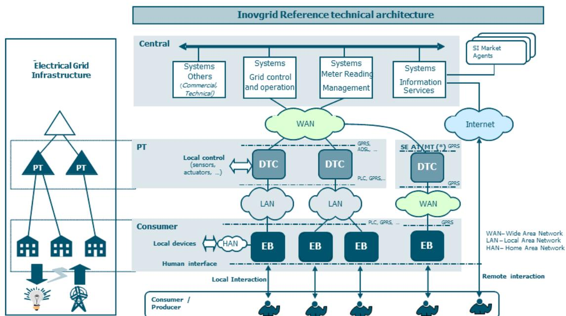
Figure 4—16: InovGrid pilot-project reference architecture
