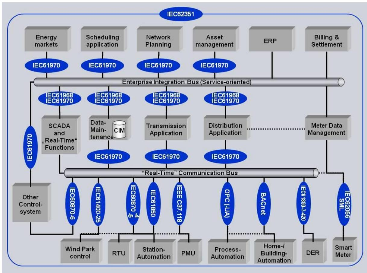
Figure 4—9: overview of the useful standards in the domain of interoperability for power utilities
