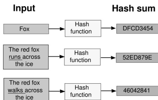
**Figure 4—25: Hash Function operation**
