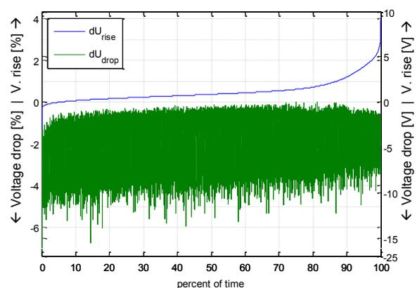
Figure 4 Duration curves of voltage rise and drop in relation to the transformer's busbar voltage (sorted according to voltage rise) in Köstendorf over one year (all operated control stages included)
