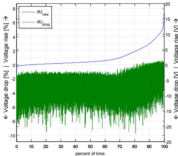
**Figure 5** Duration curves of voltage rise and voltage drop in relation to the transformer's busbar voltage (sorted according to voltage rise) in Littring over one year (all operated control stages included)
