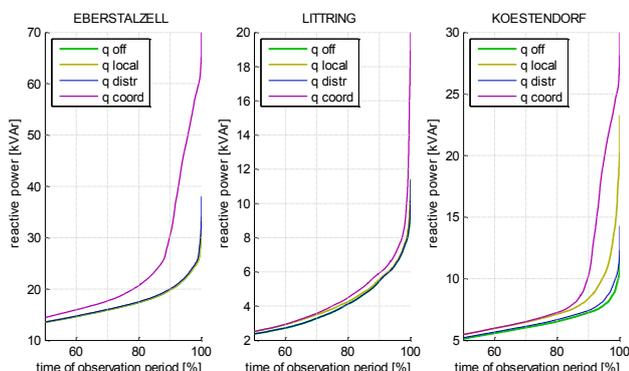
**Figure 1 Simulation results: Upper half of the duration curve of reactive power flow over the transformer in the three investigated grids (transformers' rating: 630/250 /250 kVA respectively)**
