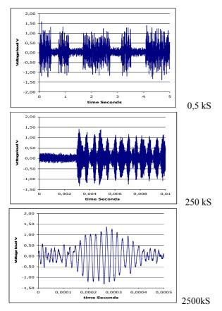
Fig. 2: Example for discontinuous signal of an AMR-PLC system
