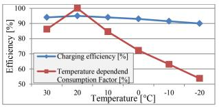
Figure 2 – Example for temperature dependency of consumption and charging efficiency
