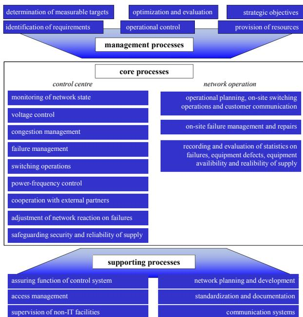
**Figure 4: Overview of processes applied in network control and operation**
